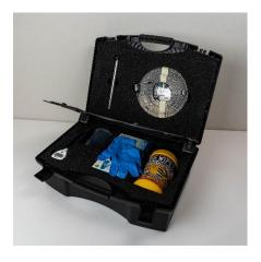
Our mission is to eliminate the need for unscheduled stops. Therefore, we include everything you need for operation, calibration, and servicing in one kit (spare sensor and tape, cleaning kit, and calibration set).
