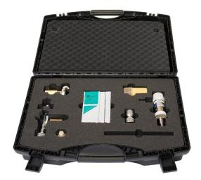
The standard kit includes the testing device (consisting of a flow regulator, flowmeter, and test tube holder) to be mounted on the compressor or cylinder. It measures CO, CO2, NOx, water vapor, and oil mist in breathing air. It also contains extra fittings and a set of tubes for testing.
