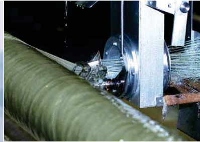
Pipe production by the cross winding method
