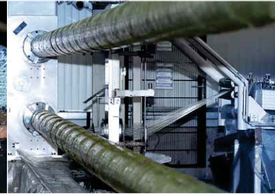
Twin winding line for the simultaneous production of two pipes
