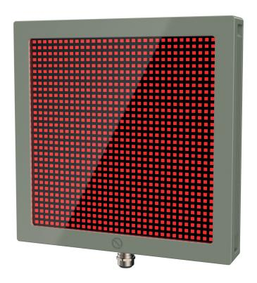
The Stop & Go Light is a large and powerful flat-shaped square signal-light with a RGB LED matrix display which can display various colors and/or symbols in the context of the Helicopter Visual Landing Aid System (HVLAS). The SGL is NVG compatible acc. to STANAG 1445. The rigid design in massive, seawater resistant aluminum is optimized for performance in extreme marine environment.
