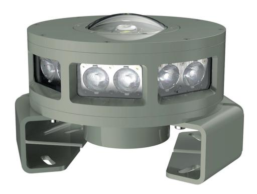
The Combined Flight Deck/Deck Edge Light (CFD/EL) is designed to mark the deck's outer limits (perimeter circle) and illuminate the entire flight deck in a way which does not dazzle pilots vision. It has a low and compact housing profile, which is made of massive seawater resistant aluminum for performance in extreme marine environments.
