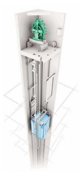
KONE MiniSpace™elevator with a small machine-room For high capacity requirements, the KONE MiniSpace™ is a highly efficient, gearless solution. The machine room for the KONE MiniSpace™ needs just 40% of the space compared with a conventional traction elevator, saving costs and maximizing the usable space in the ship.
